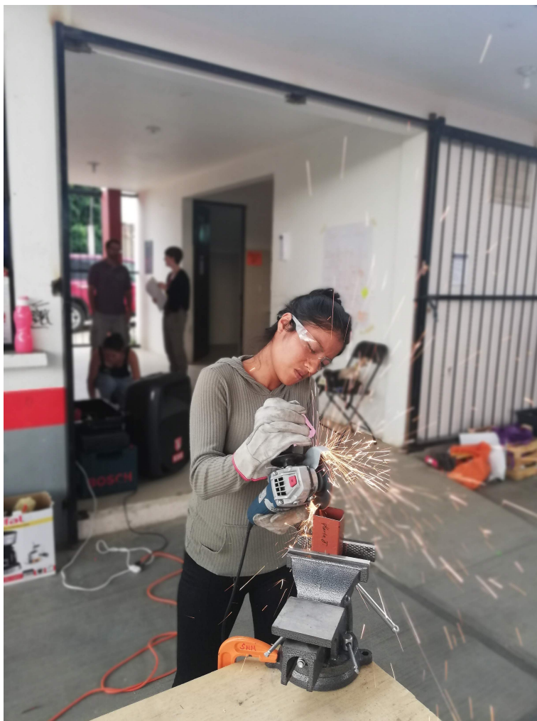
Above: A participant in DCC-Suchilquitongo cuts metal materials for her team's soil churning machine developed during the workshop.
