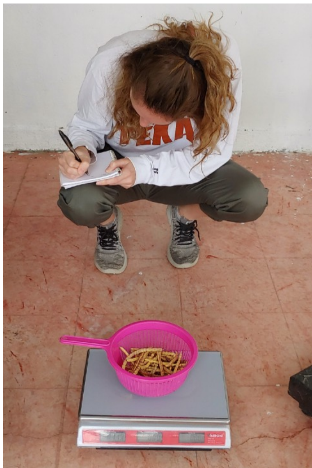
Above: PUC student gathering data on the absorption of water by mesquite pods.
